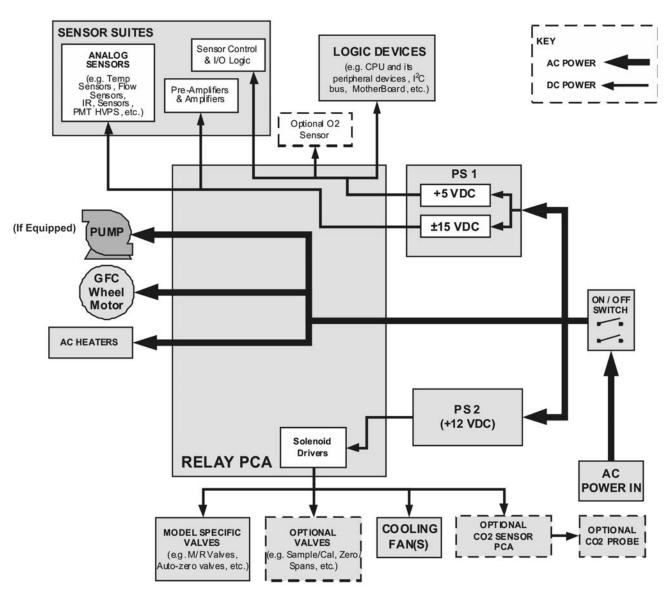
Figure 13-16: Power Distribution Block Diagram
